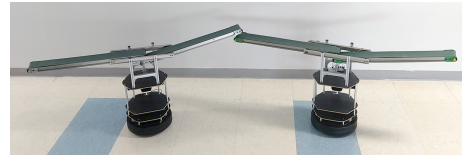
Fig. 1: A robot chain consists of three mobile conveyors.
