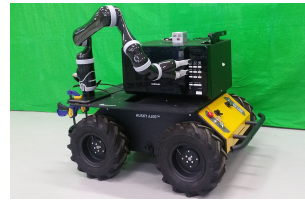
Fig. 2: A mobile microwave robot.
